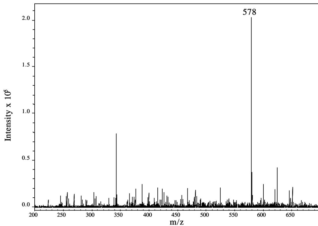
**Figure 4.4.2:** Mass spectrum of crosslinker before cleavage experiment.
