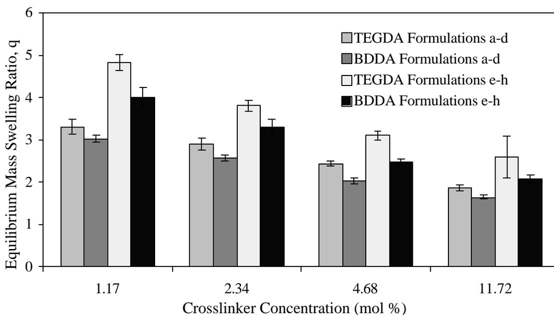
**Figure 3.5.1:** Effect of crosslinker concentration and crosslinker type on equilibrium mass swelling ratio of pHEA hydrogels.
