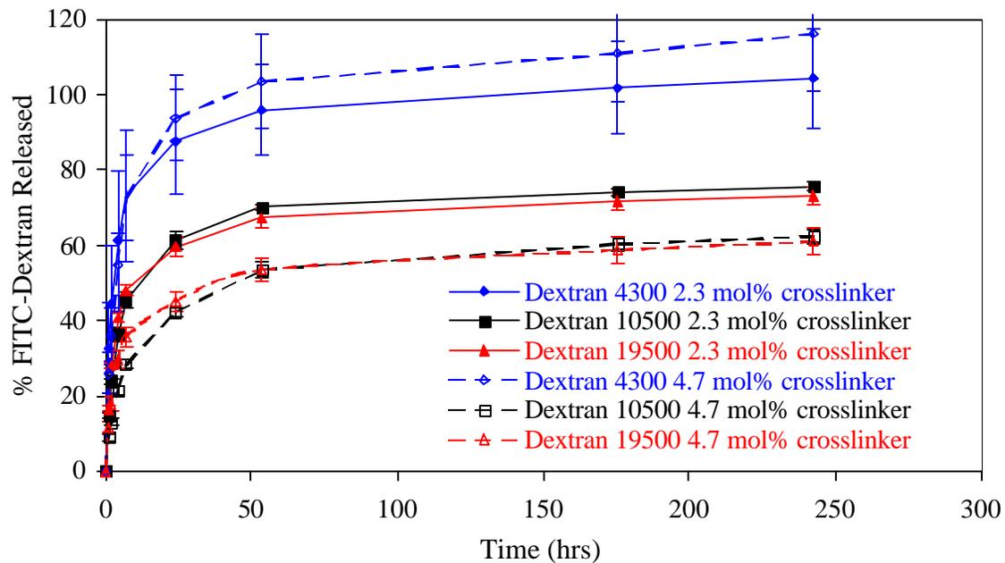
**Figure 3.4.2:** Release Study H-5. Effect of drug molecular weight and crosslinker concentration on the release of various FITC-labeled dextrans from gels made with 1,4-butanediol diacrylate.
