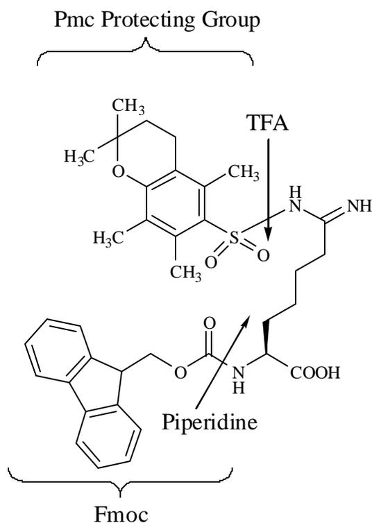
**Figure 4.2.5:** Fmoc-Arg(Pmc)-OH. Fmoc protects the N-terminus and is removed by 30% piperidine and Pmc protects the side chain and is removed with 95% TFA.
