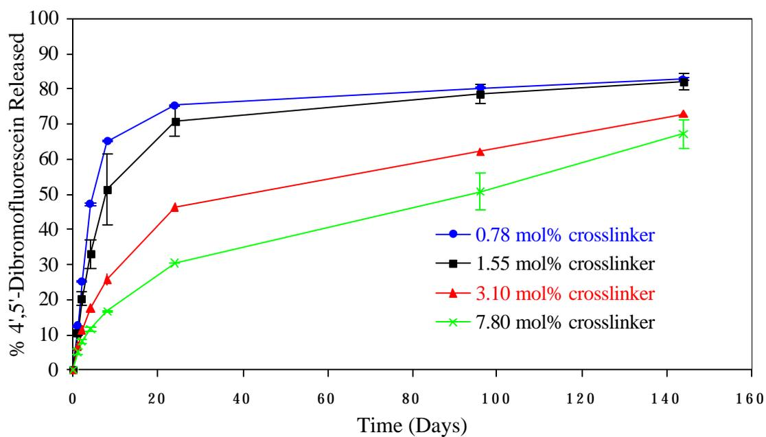
**Figure 3.3.3:** Release Study H-3. Effect of crosslinker concentration on release of 4',5'-dibromofluorescein from gels made with 1,4-butanedioldiacrylate.
