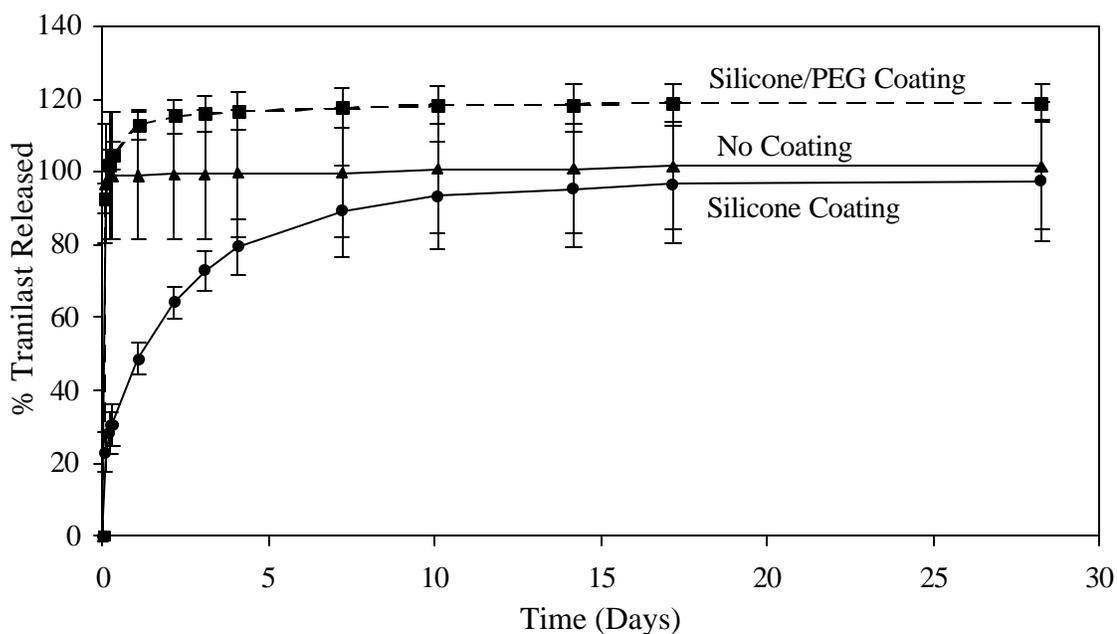
**Figure 2.4.2:** Release study R-2. Tranilast release from a reservoir with silicone coatings fabricated with or without PEG.
