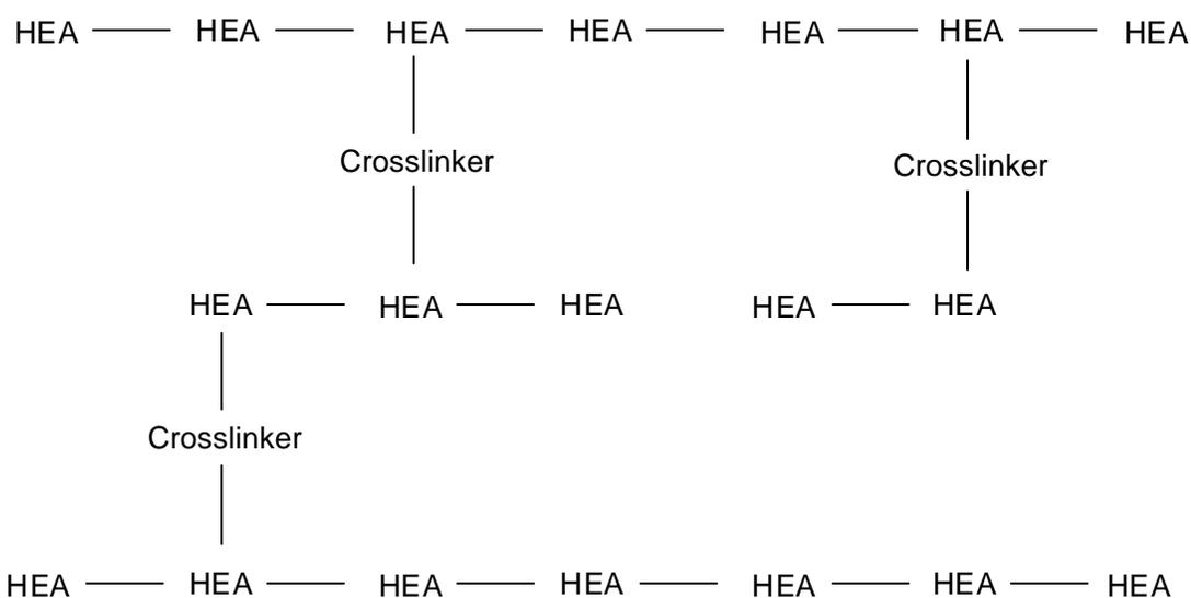
**Figure 1.5.2:** Schematic of crosslinked poly(hydroxyethyl acrylate).
