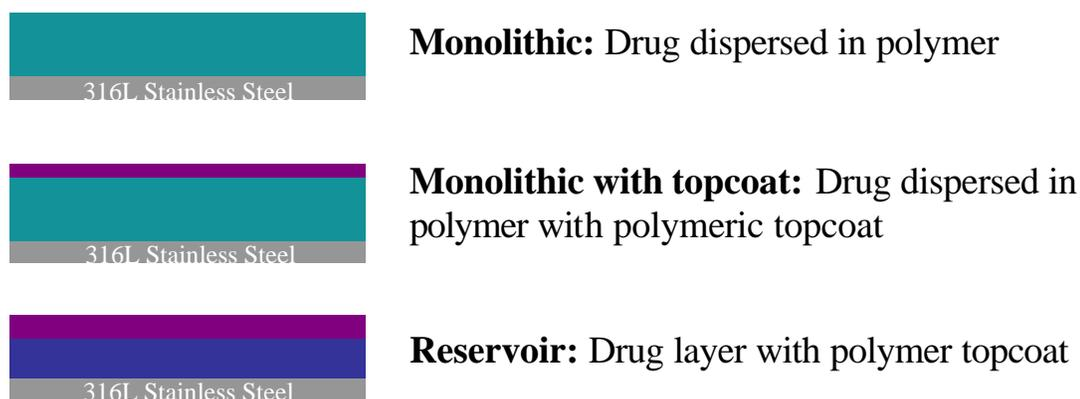
**Figure 2.2.1:** Schematic of different types of drug release coatings.
