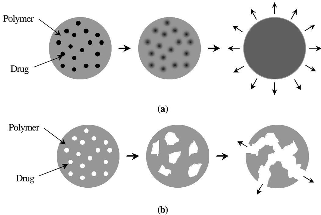
**Figure 2.1.3:** (a) Diffusion mechanism of lipophilic drugs from silicone. (b) Diffusion mechanism of hydrophilic drugs from silicone.
