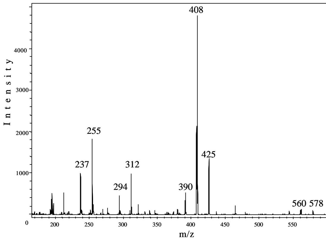
**Figure 4.3.3:** Ms/ms fragmentation spectrum of peptide crosslinker, with initial isolation of 578.
