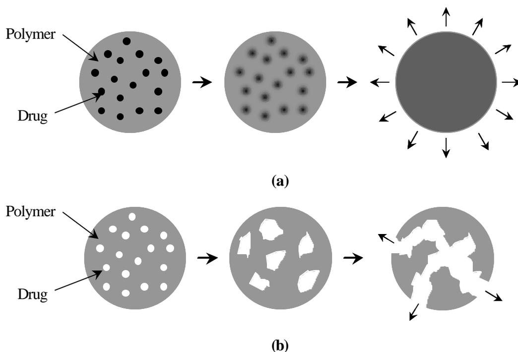
**Figure 1.4.1:** (a) Diffusion mechanism of lipophilic drugs from silicone. (b) Diffusion mechanism of hydrophilic drugs from silicone [69, 73, 75, 76].
