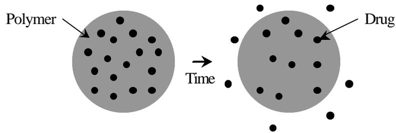
**Figure 1.3.2:** Schematic of drug release from monolithic devices.
