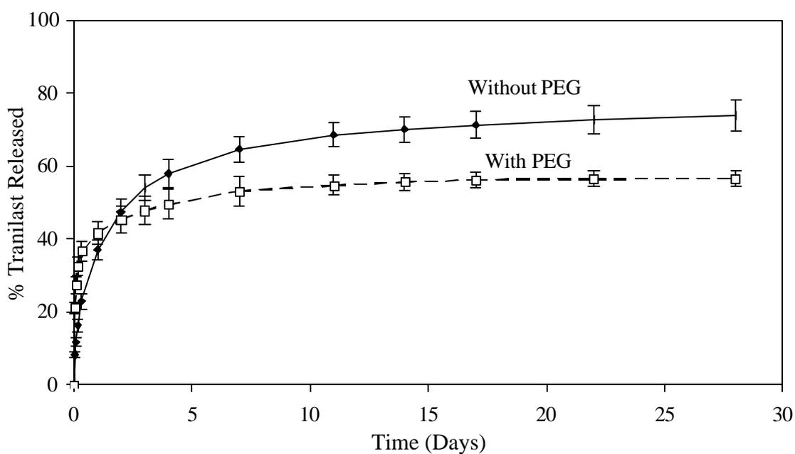
**Figure 2.3.2:** Release study M-2. Comparison of tranilast release from monolithic silicone coatings made with and without PEG.
