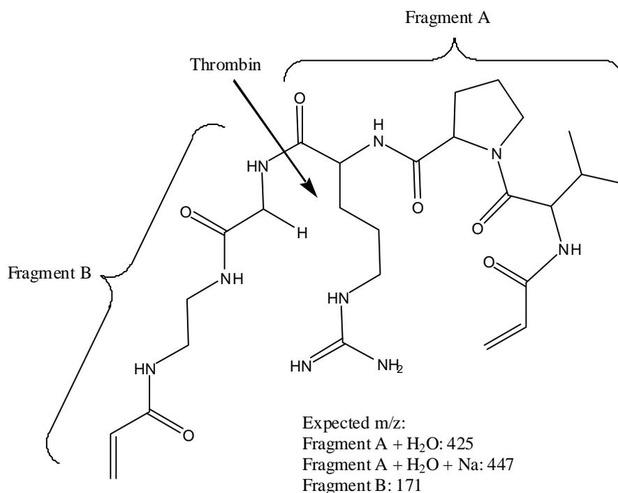
**Figure 4.4.1:** Schematic of crosslinker degradation site and products.
