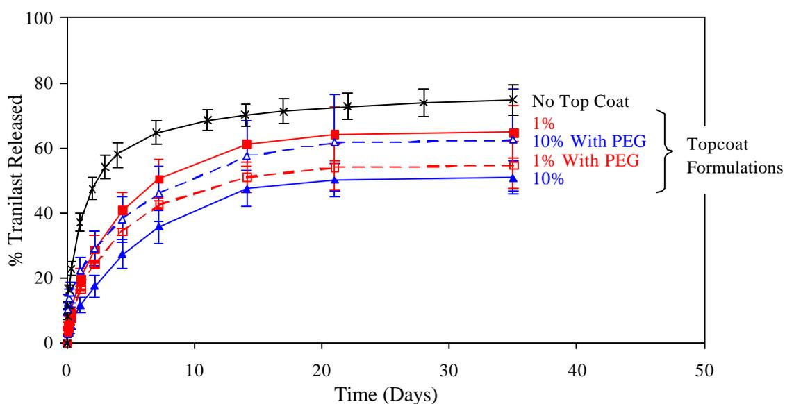
**Figure 2.3.3:** Release study M-3. Tranilast release from monolithic silicone coatings with various topcoats.
