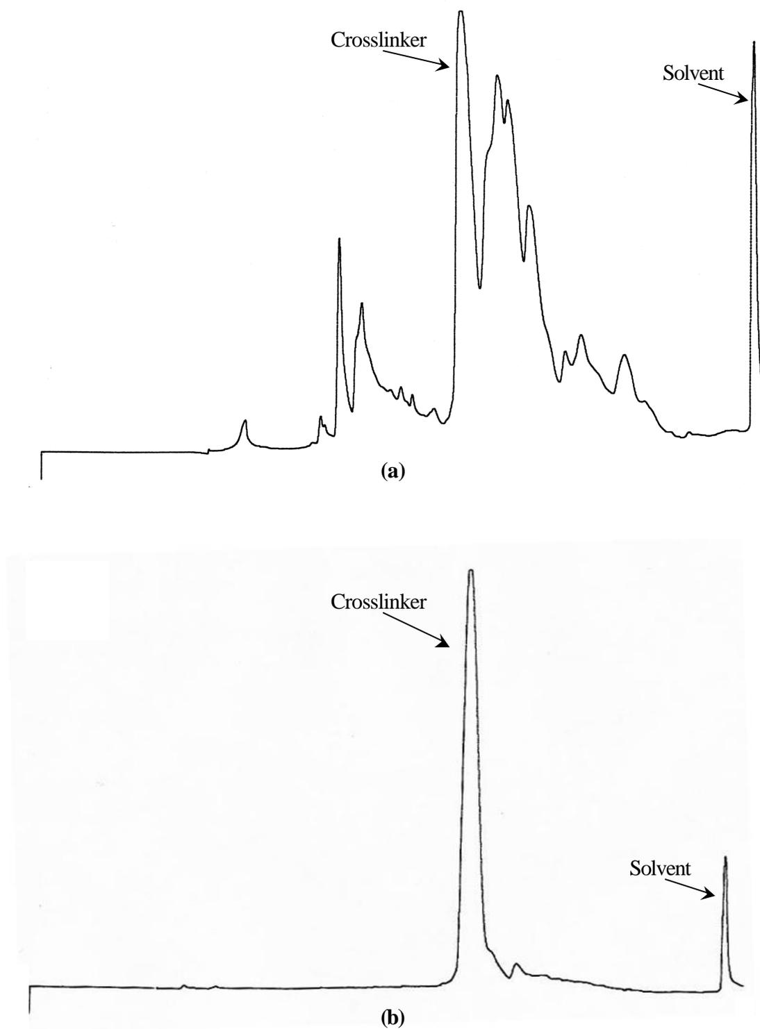
**Figure 4.3.1:** HPLC spectra of (a) unpurified and (b) purified peptide crosslinker.
