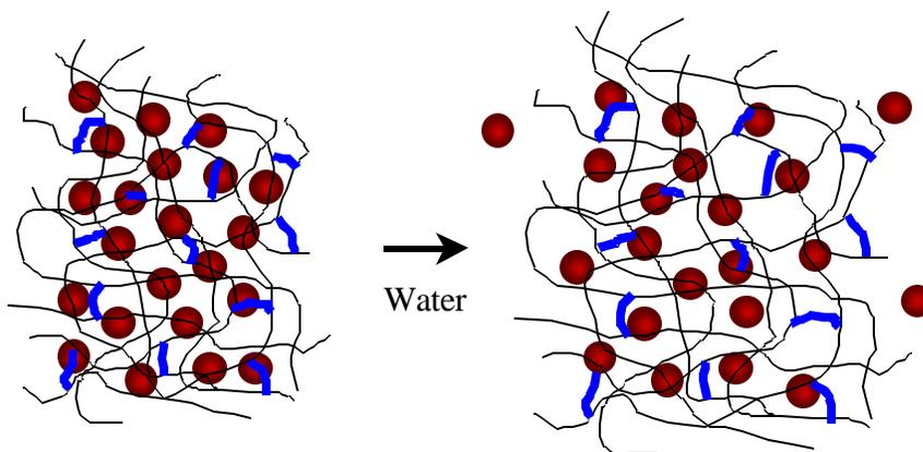
**Figure 1.3.3:** Schematic of drug release from hydrogels. Drug shown in red, hydrogel backbone shown in black, crosslinks shown in blue.
