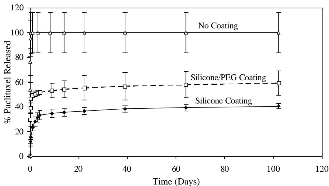
**Figure 2.4.1:** Release study R-1. Paclitaxel release from a reservoir with silicone coatings fabricated with and without PEG.
