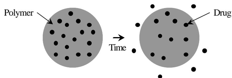
**Figure 2.1.4:** Schematic of drug release from monolithic devices.
