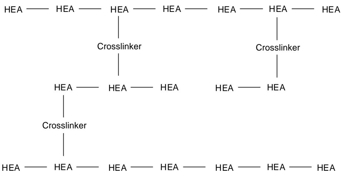
**Figure 3.1.2:** Schematic of crosslinked poly(hydroxyethyl acrylate).
