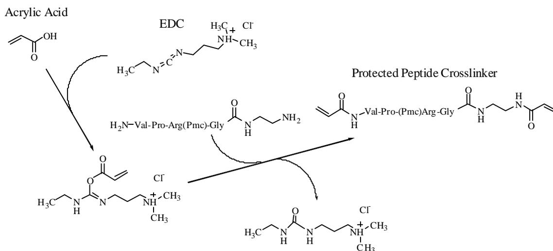
**Figure 4.2.7:** Schematic of the EDC coupling between acrylic acid and protected peptide.
