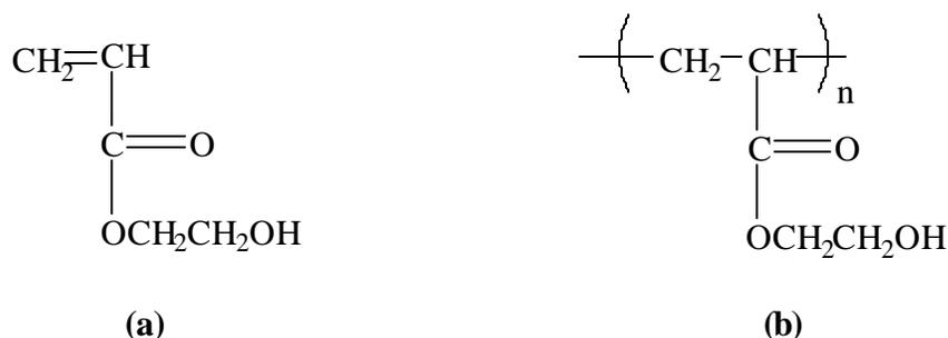
**Figure 3.1.1:** Chemical structures of (a) Hydroxyethyl acrylate monomer and (b) Poly(hydroxyethyl acrylate)
