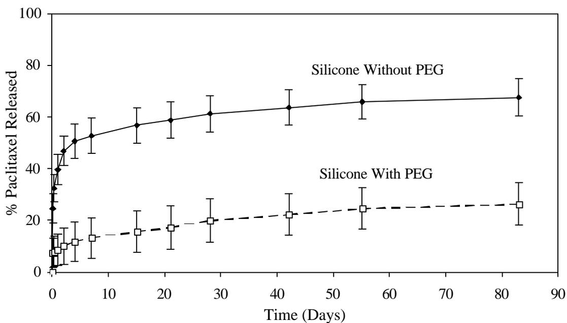
**Figure 2.3.1:** Release study M-1. Paclitaxel release from monolithic silicone coatings fabricated with or without PEG.
