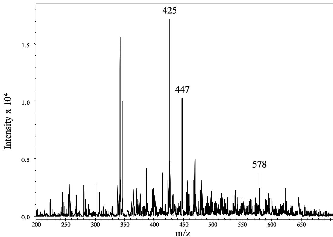
**Figure 4.4.4:** Mass spectrum of peptide crosslinker in solution with thrombin after 24 hours at 37 °C.
