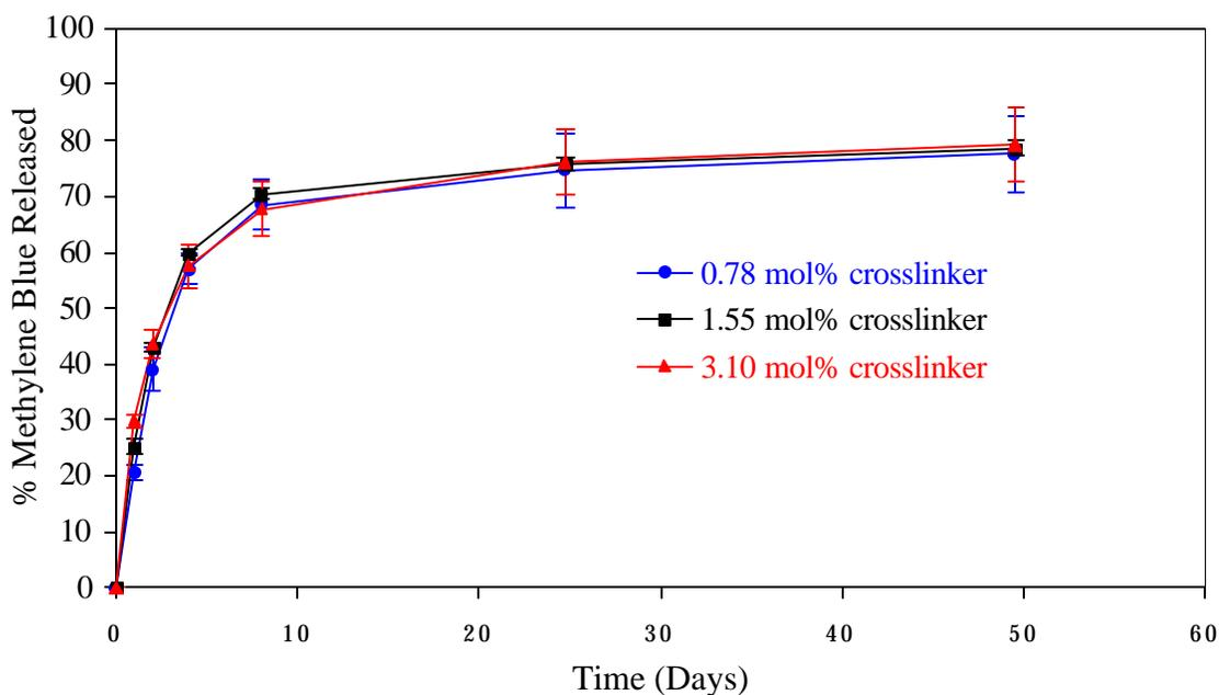
**Figure 3.3.1:** Release Study H-1. Effect of crosslinker concentration on release of methylene blue from gels made with TEGDA.
