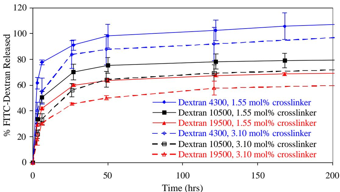
**Figure 3.4.1:** Release Study H-4. Effect of drug molecular weight and crosslinker concentration on the release of various FITC-labeled dextrans from gels made with TEGDA.
