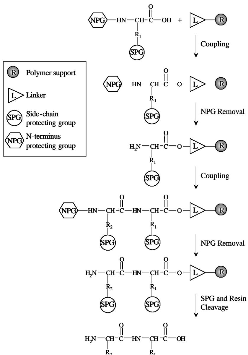
**Figure 4.1.1:** Schematic of solid phase peptide synthesis.
