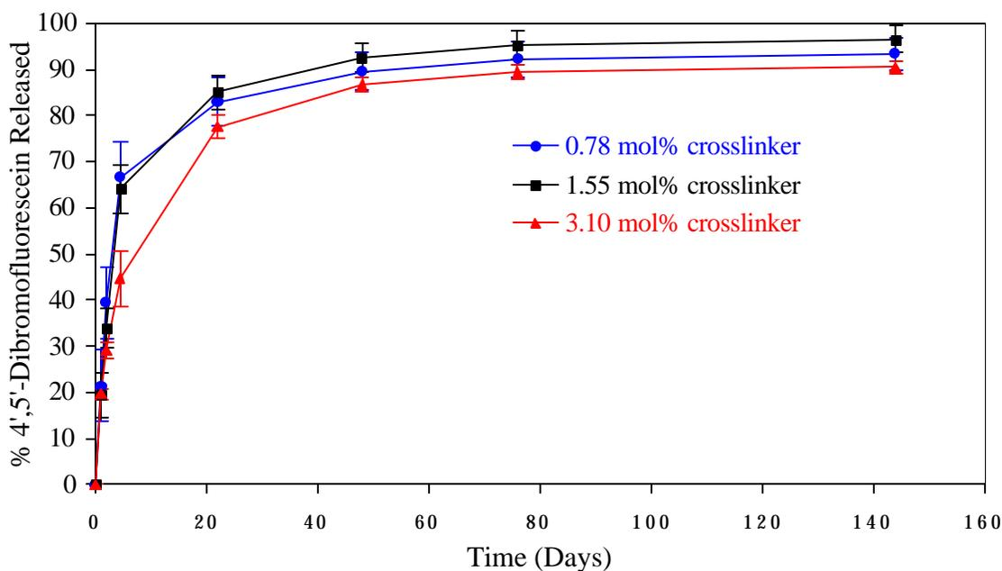
**Figure 3.3.2:** Release Study H-2. Effect of crosslinker concentration on release of 4',5'-dibromofluorescein from gels made with TEGDA.
