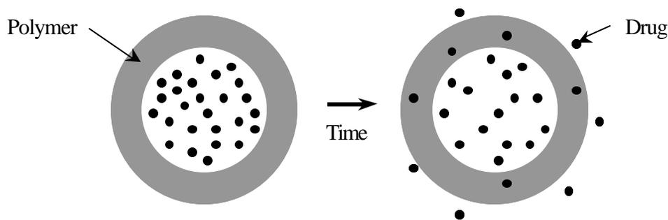
**Figure 2.1.5:** Schematic of drug release from reservoir devices.
